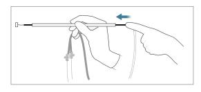
Push the *sliding tubes* completely inward. Remember to support the *filters* by taking the *connector cable* in the hand.
