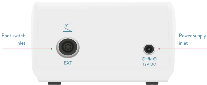
FIGURE 8: Back of the control unit console.
